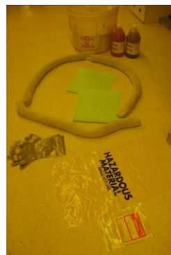
Figure 4: Contents of chemical spill kit.
