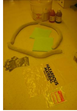
Figure 5: Contents of chemical spill kit.
