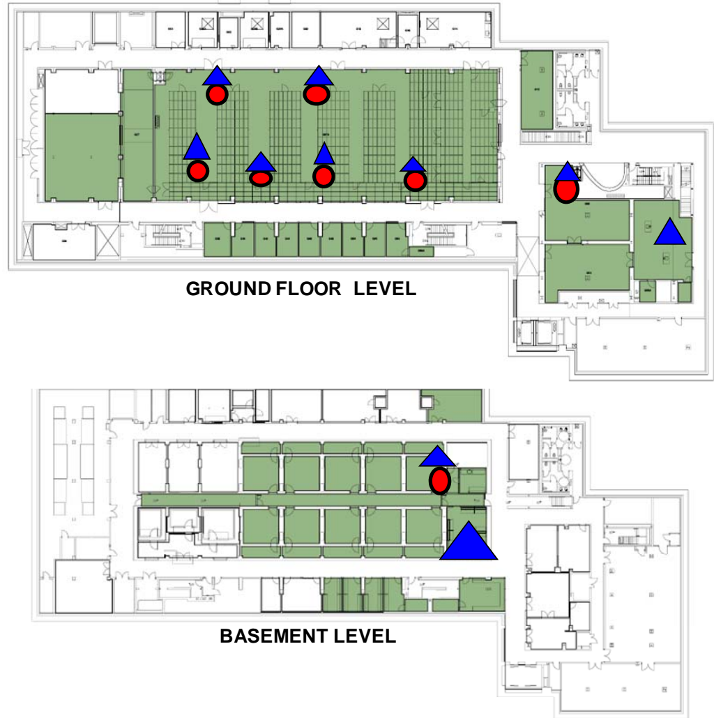
Figure 1: Locations of safety showers and eye washes.
